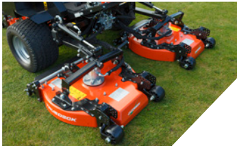
With a cutting width of 72" and a cut height of between 0.75 - 3.5", the AR321 gives you the option to cut exactly how you want.
