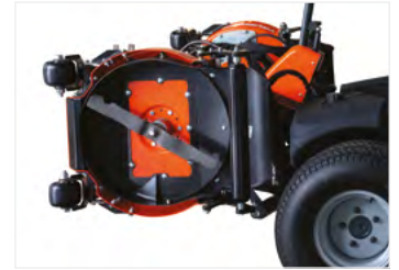
Vertical lift on outside decks for maneuverability
